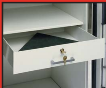
Flat Drawer With Lock Complete with handle and key lock, this drawer can be conveniently used with removable cash tray or check tray. Inside dimensions: 16 1/2" W x 3 1/4" H x 17 1/4" D Height required: 5" Installed part #13-1815
