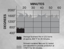
The average business fire burns at approximately 800° F. and peaks within 10-15 minutes\*\*. Schwab's insulated files are **Underwriters Laboratory** (UL) classified to provide protection at temperatures reaching 1700° F during a one-hour test. The UL label carries the
