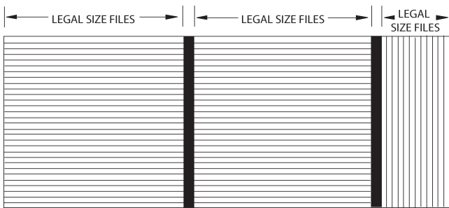
LEGAL SIZE FILING FRONT TO BACK LEGAL SIDE TO SIDE (OPTIONAL) USES HANGER BARS (INCLUDED STANDARD)
