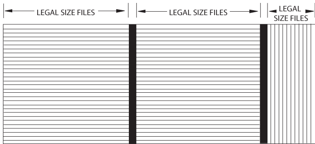
LEGAL SIZE FILING FRONT TO BACK LEGAL SIDE TO SIDE (OPTIONAL) USES HANGER BARS (INCLUDED STANDARD)
